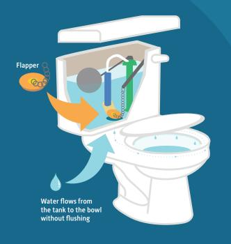
Running toilets are usually caused by water leaking from the tank to the bowl through the flapper (a rubber valve at the bottom of the tank). Toilets are the top source of leaks in homes.
