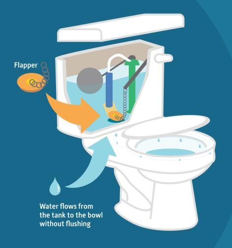
Running toilets are usually caused by water leaking from the tank to the bowl through the flapper (a rubber valve at the bottom of the tank).
